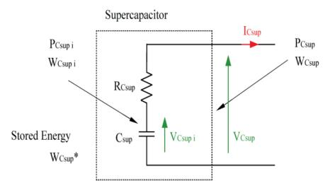
Figure 7. Model and parameter definition for power-based sizing method. Source [11].
