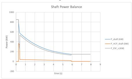
Figure 12. Power balance at the HCP shaft.
