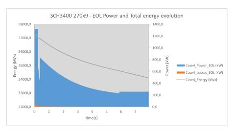
Figure 17. EOL Power and total energy evolution for case 4.
