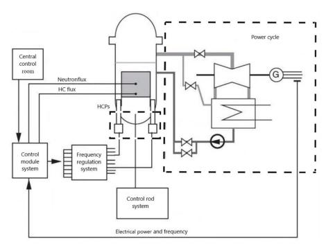
Figure 8. General scheme of the nuclear reactor with extra detail in the systems involved in the HCP control.
