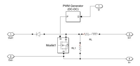
Figure 18. Booster block Simulink Model.
