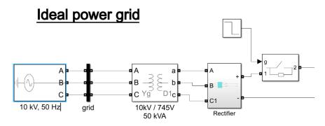
Figure 22. Ideal power grid Simulink.
