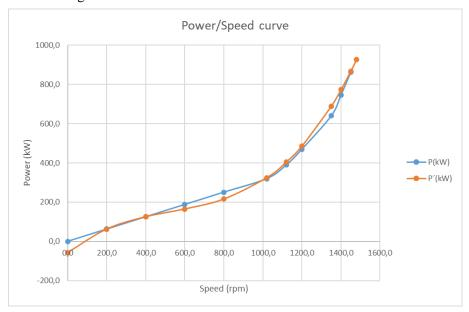
Figure 11. Power-Speed curves for the HCP motor.
