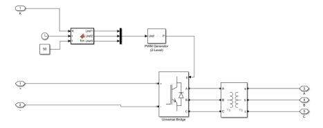
Figure 19. DC/AC Drive block Simulink model.
