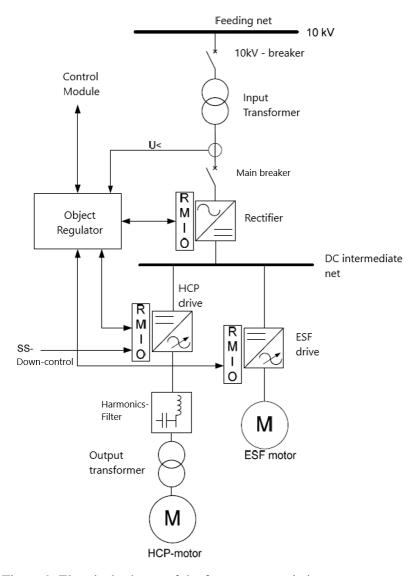
Figure 9. Electrical scheme of the frequency regulation system.
