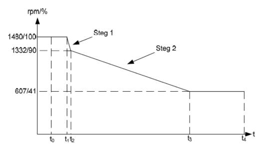
Figure 10. Ramp down speed reference for emergency stop protocols of the head circulation pumps.
