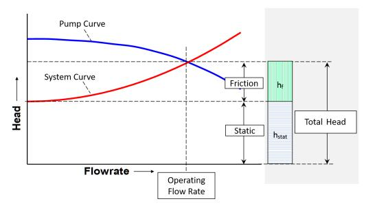
Figure 1. Pump and system curves scheme. Source [43].
