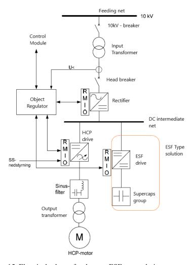
Figure 15. Electrical scheme for the new ESF type-solution.
